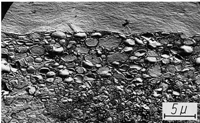
Fig. 2. Open-porous top region of VCVA copolymer film, covered by epoxy resin layer that has penetrated into the microvoids.
